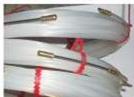
Guiding head with spring
